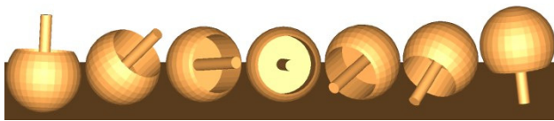
Figure 20: Snapshot of Tippe Top inversion, from left to right
