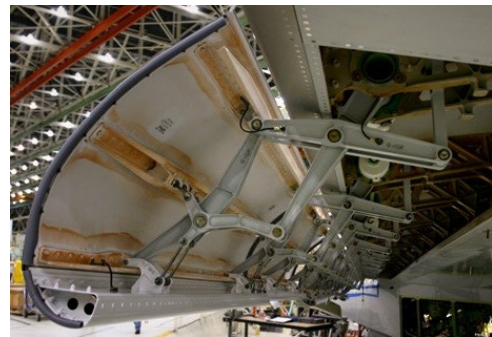
Figure 21. Wing variable camber leading edge flap
